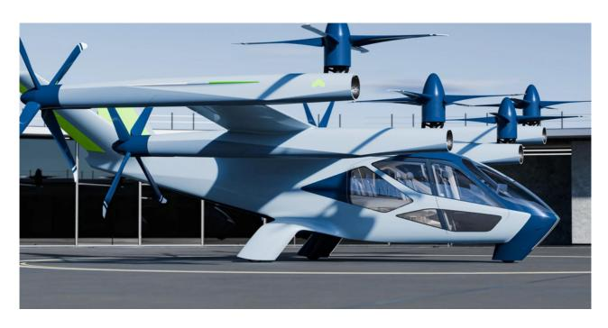
The S-A2 is designed to meet typical urban operation needs with flights ranging from 25 to 40 miles, cruising at a speed of 120 miles per hour at an altitude of 1,500 feet. The vehicle features a distributed electric propulsion architecture and eight tilting rotors. It is designed to operate as quietly as a dishwasher during vertical takeoff and landing phases, and even more quietly during horizontal flight.
